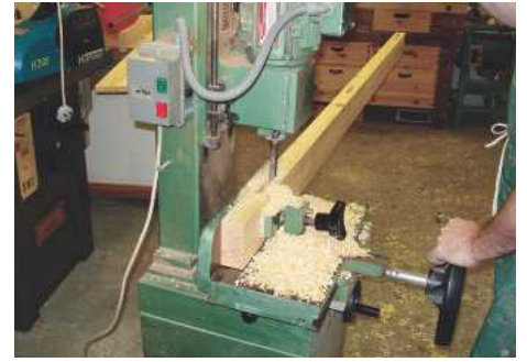
▲ Pic.3 ...which Mike cut on the mortiser using a 12mm chisel, saving his chisel and mallet...
